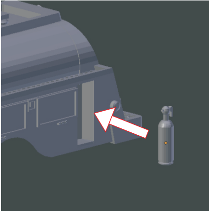
Step 2 - attach the fire extinguisher to the tanker bed
