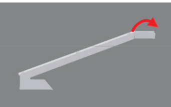
Step 4: bend the narrow end of the boom down as shown on left
