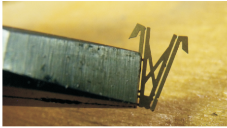
Step 1: grip the boom with pliers
